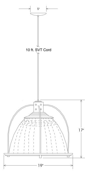
16" Acrylic Prismatic/Ribbed Hanging Dome with bars and prismatic lens closed bottom, on SVT cord, 19" diameter, 17" high, one 200 Watt maximum incandescent bulb or HID 200 Watt maximum (bulb not included), Painted finish, UL Listed, Weight 8 lbs
